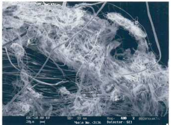
Figure 6: SEM photograph of exfoliated yarn unraveled from fabric (Magnification= 400 x 00209060257)
